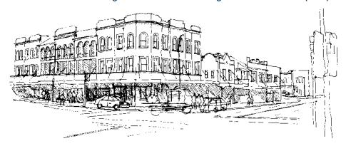
**FIGURE 19** Roof design – Roof forms must be contained within the building envelope. Varying roof forms including hips, gables, flat roofs and parapets are encouraged in the Transition Areas
