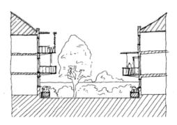
**FIGURE 48** Vegetation and balcony screening must be used to enhance privacy when the recommended separations are not able to be achieved.
