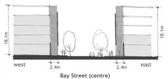
Indicative existing built form Articulation zone Design colonnades including the size and spacing of the columns integral with the building design and with regard to adjoining colonnades if they exist
