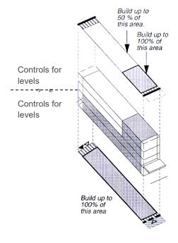
**FIGURE 20** 3-dimensional controls Highlighting the building envelopes.
